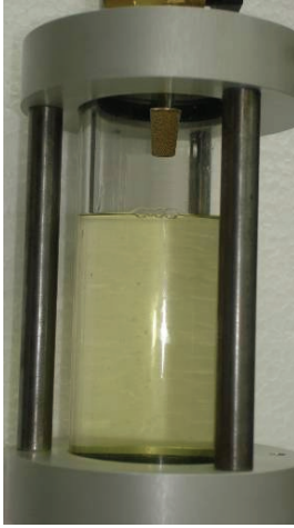
Oil and refrigerant well mixed with each other.
