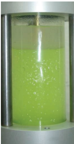
Refrigerant/UV mixture fouled by water.
