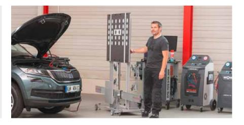
Adjustment of the calibration board holder for camera calibration by means of spring balancing.
