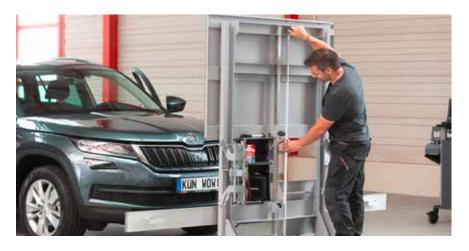
Adjustment of the laser carrier for radar calibration (up to 1.0 m).
